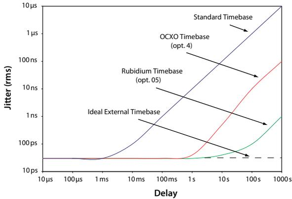
Jitter vs. programmed delay
